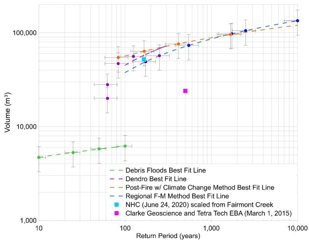
Figure 3-1. The frequency-volume methods considered reasonable for Cold Spring Creek. Best fit lines are trimmed at the 100-year return period as BGC considers debris flows below that return period are unlikely. The figure also shows the Clarke Geoscience and Tetra Tech EBA (March 1, 2015) F-M estimate as well as the recently updated (NHC, June 24, 2020) estimate for Fairmont Creek adjusted by watershed area. Error bars are based on judgement.
