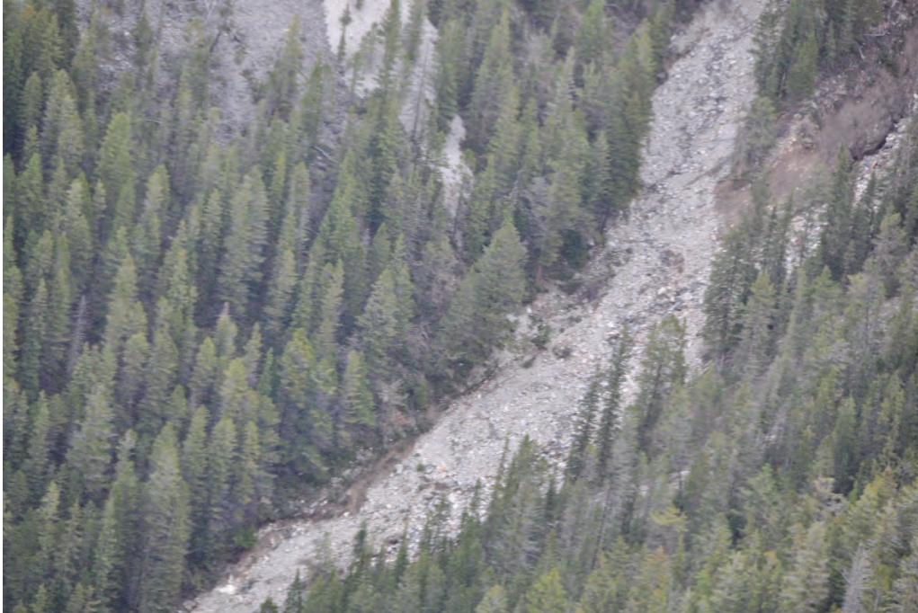
Photo 3.1 Sediment tracks and debris 300 m upstream of the ski hill water intake on the north tributary of Fairmont Creek. A debris flow deposit in the forest is visible in the top center of the image while extensive deposits of sediment in the two main channels are also visible.
