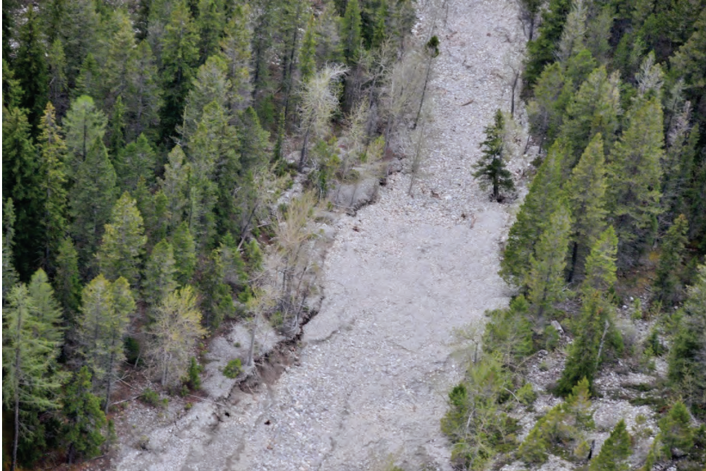
Photo 3.5 Middle tributary approximately 700 m upstream of confluence with main channel. Debris flow deposit with no identifiable channel Indicates that mass movement processes dominated the transport of material in this region of the creek.
