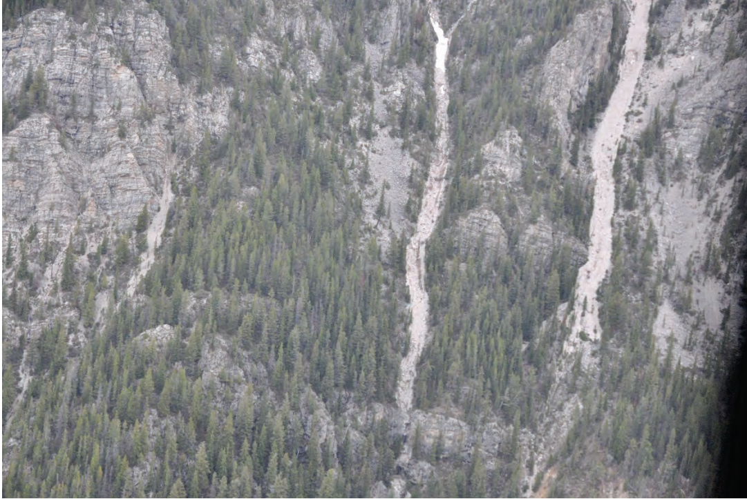
Photo 3.37 Upslope debris flow channels that merged and then enter Cold Spring Creek at the location shown in Photo 3-36.
