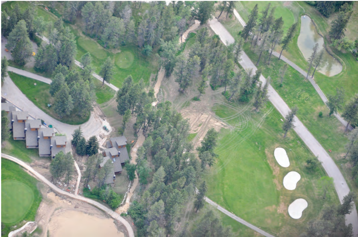
Photo 3.31 Golf course sediment containment pond and area downstream that experienced clearwater flooding. Flood waters went overtop of the paved golf course road.
