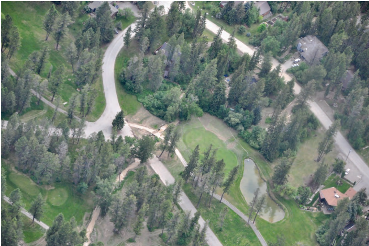
Photo 3.35 Aerial image of Fairmont Creek downstream of golf course sediment containment pond. Roadway in image center and top of image were overtopped during the event.
