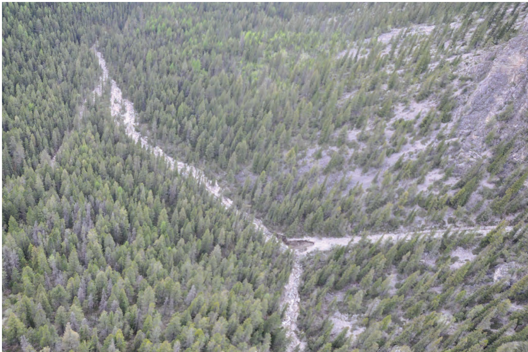
Photo 3.36 Major debris flow system on Cold Spring Creek located 5.7 km upstream from the dam can be seen on image right. The toe of the deposit has been scoured by river flows.
